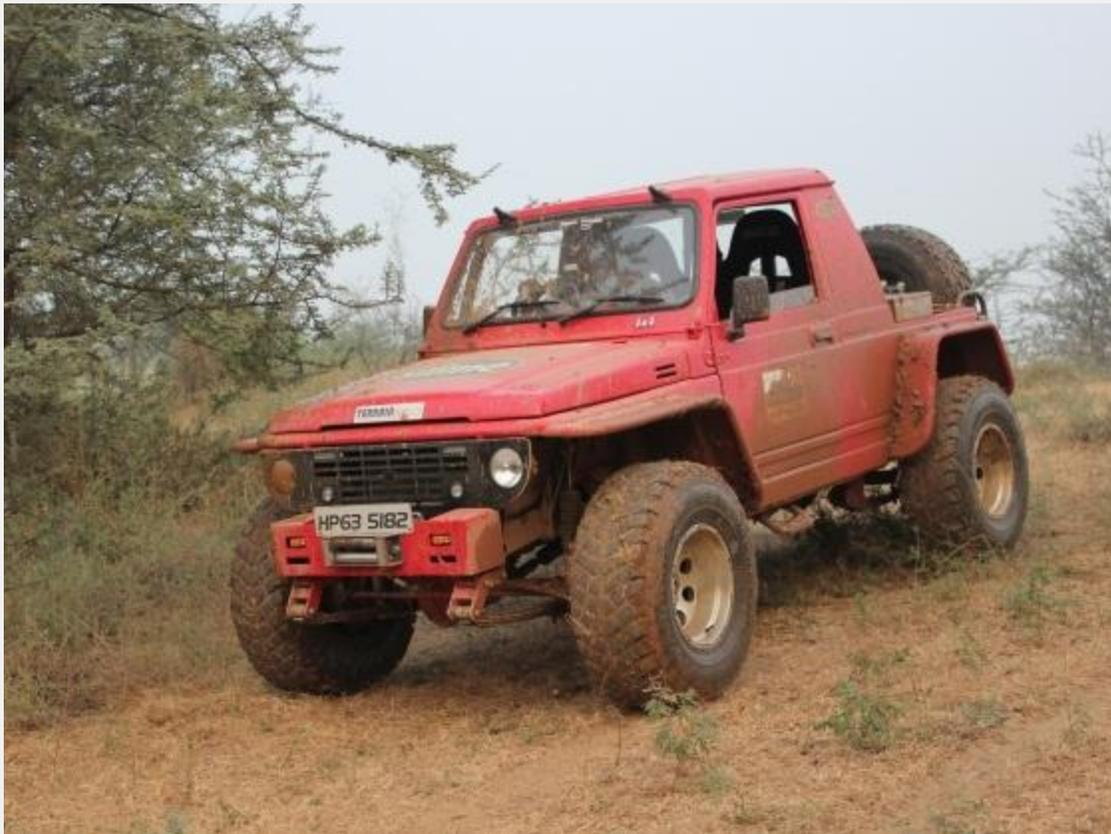
A stand-out was a fully modified off-roader owned by Sumeer Tandon called 'The Monster'. Built on a Gypsy frame with the cylinder head from the existing and a modified differential lock, with a Maruti Baleno engine, Sparco racing seats, numerous buttons for various controls and more.
